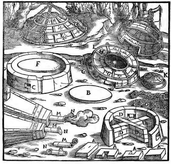
A—RECTANGULAR STONES. B—Sole-stone. C—Air-holes. D—Internal walls. E—Pome. F—Crucible. G—Bands. H—Bars. I—Apertures in the dome. K—Lid of the dome. L—Rings. M—Pipes. N—Valves. O—Chains.
